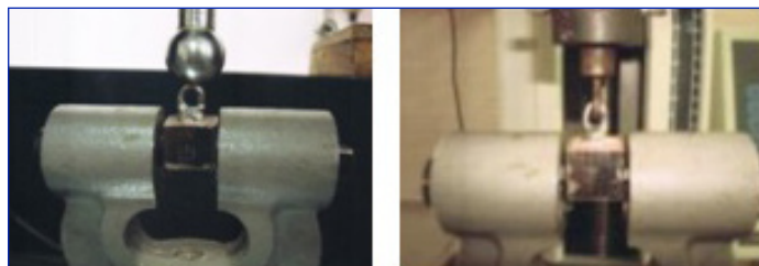
[Table/Fig-3]: Crowns subjected to an axial dislodgement force until failure on a Universal Testing Machine (Instron) at a cross head speed of 0.5 mm/min
